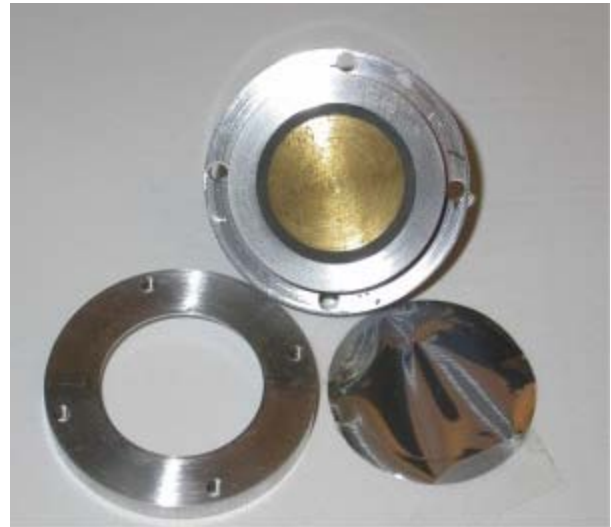
Components of an oscillating super-leak transducer. The plastic film with micrometre-scale holes is shown in the lower right corner. Image: Zach Conway.
