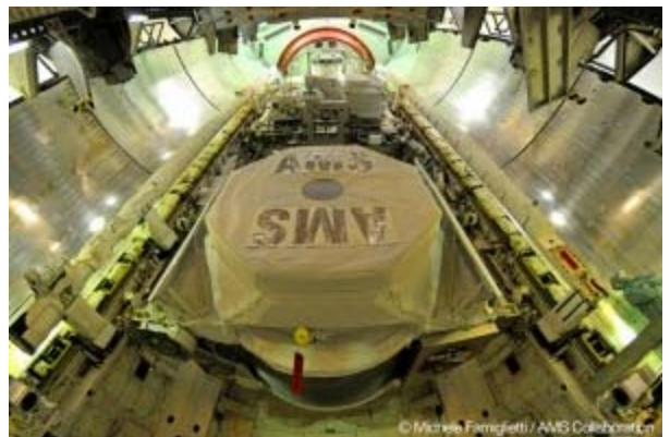
AMS-02 loaded into the shuttle bay. Image: Michele Famiglietti / AMS-02 Collaboration
