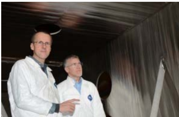
PAVAC President Ralf Edinger (left) and associate Doug LaPointe inspect a vacuum chamber the company is manufacturing for an electron beam welder. Image: Ralf Edinger
