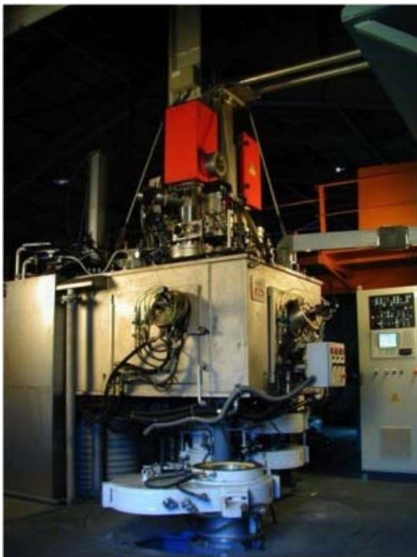
One of the seven electron beam melting furnaces at Tokyo Denkai. Image: Tokyo Denkai Co., Ltd.
