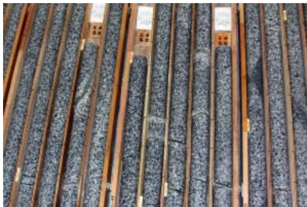
Sample borings of the granite rock from the northern site in the mountains in Iwate prefecture
