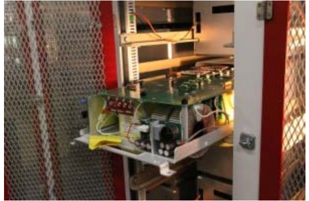
One cell of the Marx P2 modulator. In developing their second Marx modulator prototype, SLAC scientists outfitted each cell, or building block, with more system control capabilities. This approach increases the number of fail-safes in the system and therefore its overall reliability. Image: Ray Larsen
