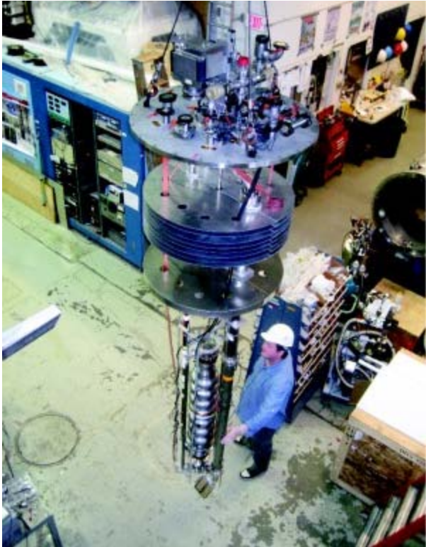
Cornell's first ERL cavity during its vertical test showing the required small energy loss. Image: Cornell / LEPP
