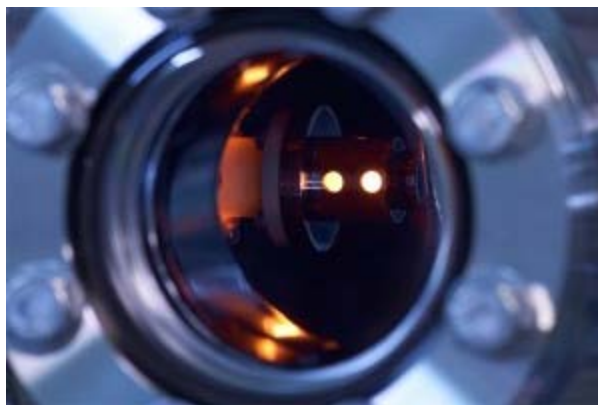
RF gun for the Quantum Beam Project at KEK. The cathode substrate, made of molybdenum, is being heat-processed for cleaning its surface. Image: Nobu Toge
