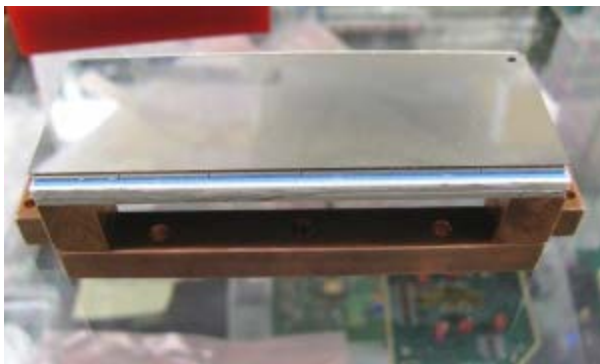
The current, most recent module of the "Helmholtz cube" that uses 3-D technology and the latest bonding techniques.
