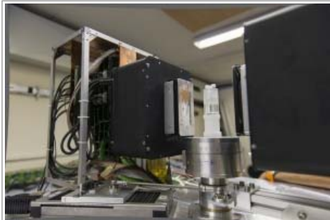
Snapshot of a "phantom", a test object, surrounded by the AX-PET photon detectors.
