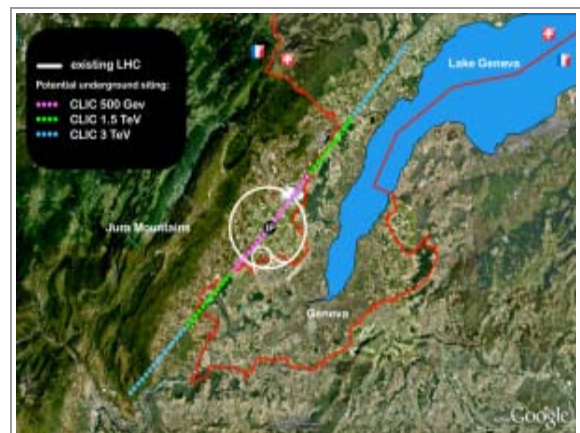
Image 2: Possible CLIC location, showing the three energy stages.
