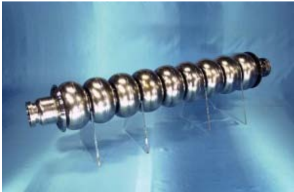
A one-metre-long nine-cell ILC SCRF niobium cavity.
