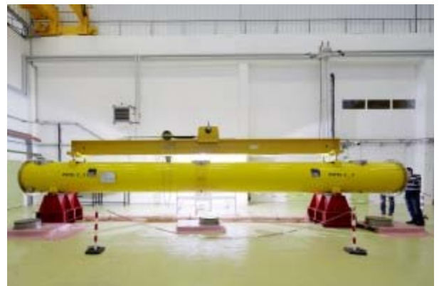
Having a good look at cryomodule production: an industrial study produced interesting results. Pictured: a cryomodule for the European XFEL under construction at CEA Saclay. Image: DESY / Heiner Müller-Elsner.
