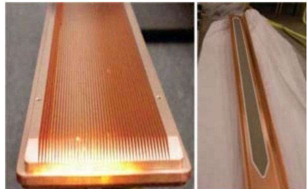
Mitigation techniques include using grooved chamber surfaces (left) in the dipoles and clearing electrodes (right) in the high-field wigglers.
