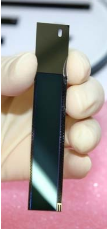
Figure 2: Photograph of mechanical sample of a thin, self-supporting DEPDET ladder
