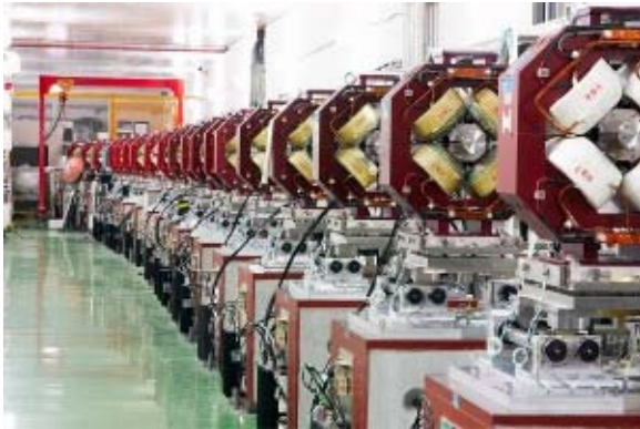
These quadrupoles at the ATF2 test facility at KEK in Japan get the beam down to the required size. Image: KEK
