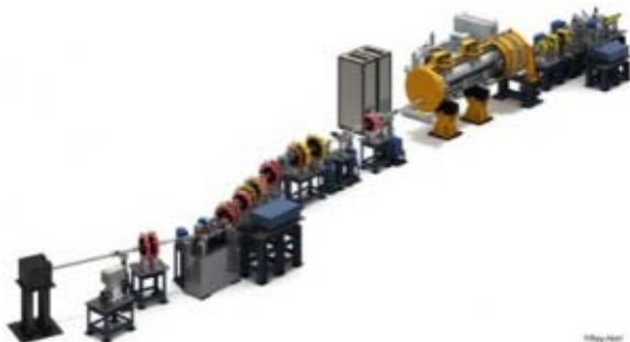
Illustration of the superconducting accelerator (on the right), the beam line for squeezing its transverse size (middle), and the X-ray generation section (on the left) that operates through the collision of the accumulated laser power in the four-mirror optical cavity and using a squeezed electron beam.
