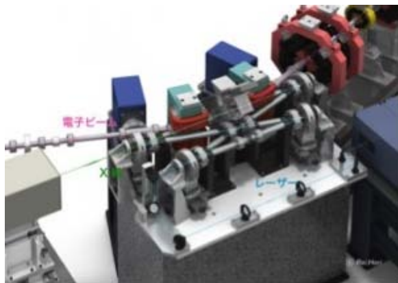
Illustration of the four-mirror optical cavity with laser axis (blue lines). An electron beam comes in from the right to the left (pink lines), and collides head-on with the laser beam inside of the four-mirror optical cavity. The generated X-rays leave to the left (green line).
