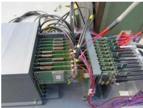
Close-up of the technological prototype that was successfully tested with power pulsing in a magnetic field as well as with beam.
