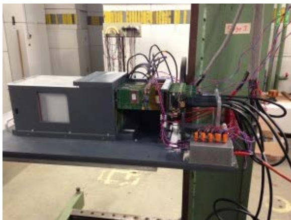
Complete setup of the SiW-ecal test in the test beam. The small silver box makes sure that the power pulsing works.
