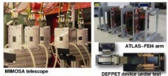
These are the components of the combined beam test: the MIMOSA telescope, the ATLAS-FE14 arm and the DEFPET device under test.
