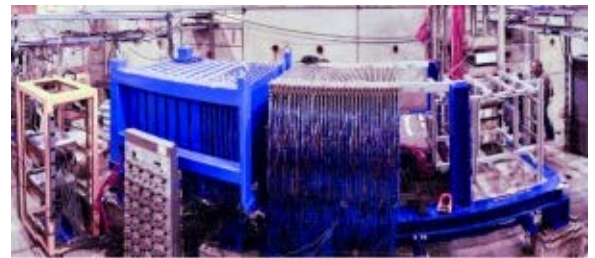
The prototype of the tungsten digital hadronic calorimeter for CLIC.
