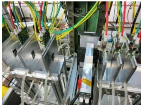
Under scrutiny in the DESY test beam with the help of the beam telescope: timepix chips.
