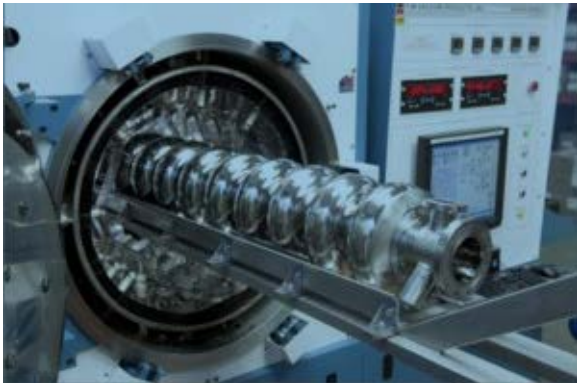
An SRF cavity entering the furnace where it will be baked with nitrogen or argon. Photo courtesy of Anna Grassellino
