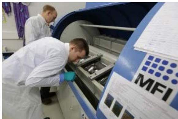
Using different polishing materials, ranging from centimetres to millimetres in size, the cavities are refined in a type of tumbler. Images: DESY/Dirk Nölle
