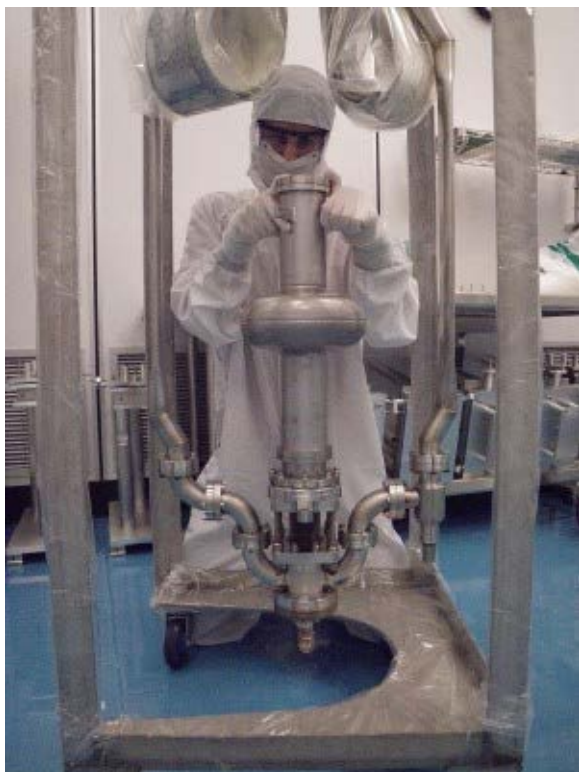
Sam Posen assembles a Nb 3 Sn cavity to a test stand in the clean room. Image: Cornell Laboratory for Accelerator-based Sciences and Education (CLASSE)
