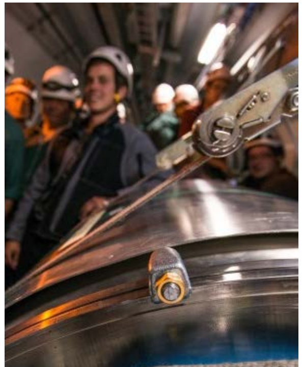
With the closure of the last of 1695 magnet interconnections in June, the LHC is getting ready for the cooldown. Some of the pre-accelerators are already back in service. Image: CERN
