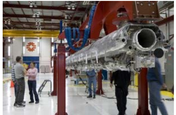
Early on, the U.S. high-energy physics community built an infrastructure to accommodate the large scale of the International Linear Collider. Pictured here is an ILC-type cryomodule at one of Fermilab's Industrial Complex buildings. Jefferson and SLAC laboratories, as well as institutions such as Cornell University, were a part of the U.S. infrastructure for ILC SCRF. Credit: Fermilab
