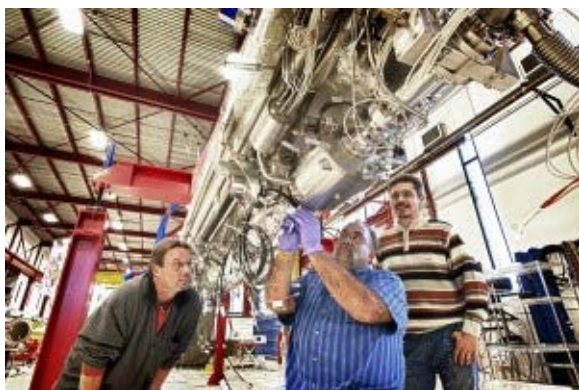
CM2 cryomodule being assembled at Fermilab's Industrial Center Building (2011). Photo: Reidar Hahn
