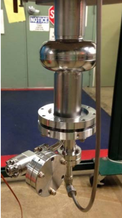
A team from Fermilab's Accelerator Division has successfully powered this small SRF cavity with a magnetron. Now they aim to power a large, application-specific model. Photo: Brian Chase, Fermilab
