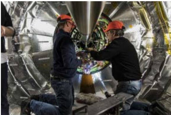
The luminometer was installed in the CMS detector in January. Image: CERN
