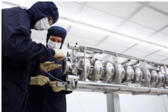
Cavity production at Zanon in Italy. Image: DESY, Heiner Müller-Elsner
