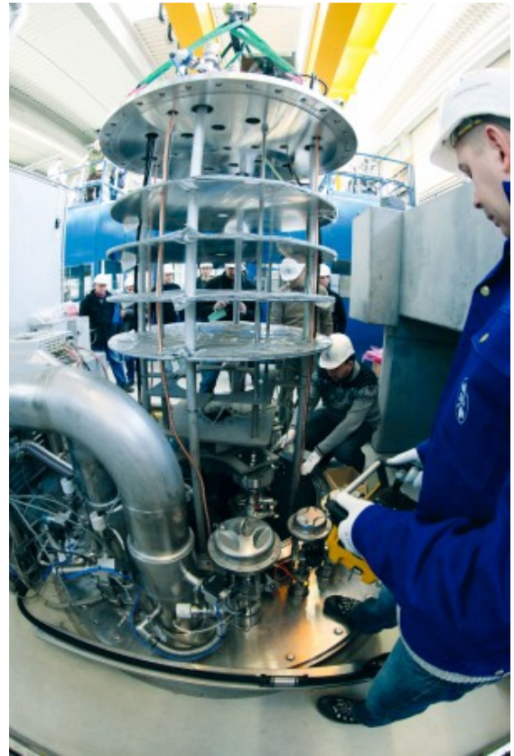
One of two cryostats for vertical cavity tests in the AMTF hall.
