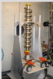
Last week US facilities reached a milestone in testing superconducting cavities for the ILC.
