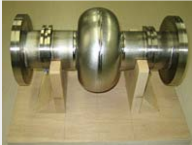
The first Korean 1.5 GHz SRF cavity for ILC R&D.
