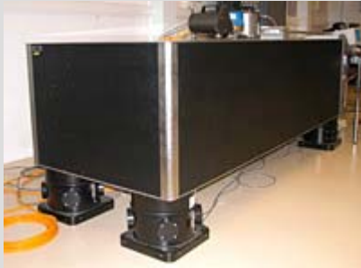
The 731-kilogramme stabilisation table at Anncy, with its active feet.
