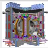
A cutaway view of ITER, a large international project to demonstrate the scientific and technological feasibility of fusion.
