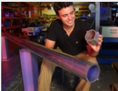
Mauro Pivi holds a section of beam pipe with built-in grooves. (Image courtesy of Brad Plummer.)
