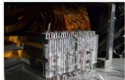
Prototype of an electromagnetic calorimeter.
