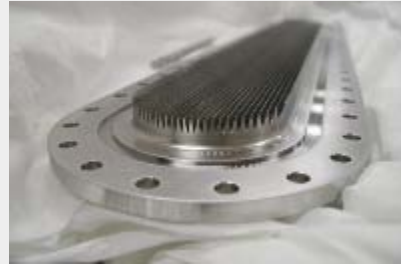
This insert, manufactured by SLAC and the company EMEGA, was placed inside the KEK-B accelerator beam pipe to trap stray electrons with its triangular grooves. Photo: Mauro Pivi.
