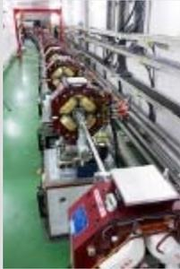
The Accelerator Test Facility 2 in Japan uses a 50-meter series of magnets to focus its electron beam. (Photo by N. Toge, KEK)
