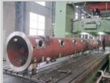
Vacuum vessel fabrication in factory
