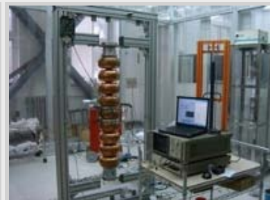
Field flatness measurement and adjusting (reached flatness of 98%)
