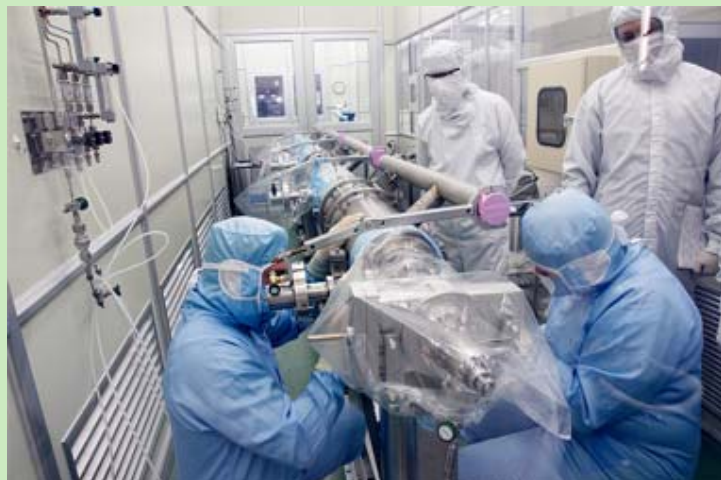
The cavities being string-assembled by technicians from DESY and Fermilab, in the KEK's ISO Class-4 clean room. (Photo by Nobu Toge)
