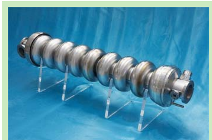
The one meter-long superconducting accelerating cavities are made from nine cells, polished to provide micro-level surface smoothness, and free of impurities. A series of detailed chemical treatments and processes make the cavity literally sparkle. (Photo by Nobu Toge)
