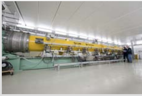
Cryomodule 1 is the only eight-cavity SRF cryomodule in the United States. It was successfully cooled to 2 Kelvin (-271° C) on Nov. 22. Photo: Reidar Hahn
