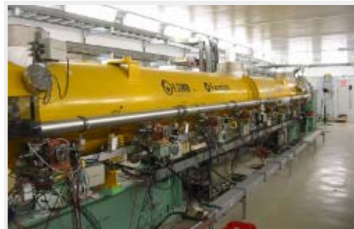
The first cryomodule at Fermilab, called CM-1 (a collaboration of Fermilab, DESY, INFN) in the superconducting radiofrequency accelerator test facility has recently been cooled down to 2 kelvins for testing
