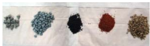
Medias are tumbled inside the niobium cavities. The grey cones (far left) are a plastic with aluminum silicate, used for bulk removal. The powder blue media (second from left) are
