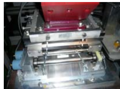
The quadrupole magnet sits on the mover, but one of wires was cut. The earthquake-proof apparatus worked as designed. Image: Nobuhiro Terunuma
