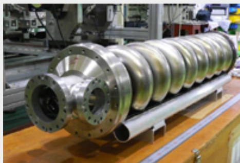
TESLA-like 9 cell cavity will soon be tested in a vertical cryostat for gradient performance.
