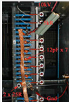
Prototype PSI kicker stack adapted for ILC kicker "proof of principle" test bed.
