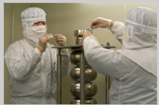
Fumio Furuta, KEK, and Hyong Suk KIM, Kyungpook National University, prepare a 9-cell ICHIRO cavity for high gradient field test in the clean room of STF, KEK.
