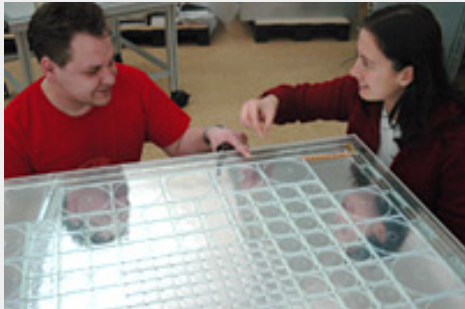
Erika Garutti and a technician, Oleg Chernyshov, checking the "eyes" of the seventh layer for the prototype of the hadron calorimeter, an essential part of future ILC detectors.
