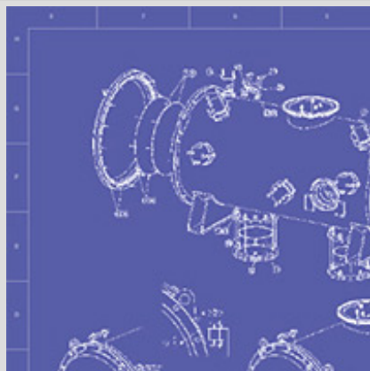
Assembly drawing of a test cryostat for superconducting RF cavities (Image: Clark Reid, Mayling Wong, and Valeri Polubotko)
