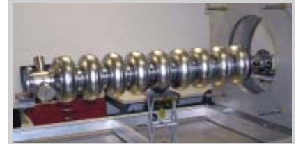
So far US industry has produced five cavities for ILC R&D. (Image courtesy of Advanced Energy Systems)
