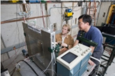
University of Texas student Jacob Smith (left) and his advisor Jae Yu assemble the GEM chamber in the Meson Test Beam Facility.
