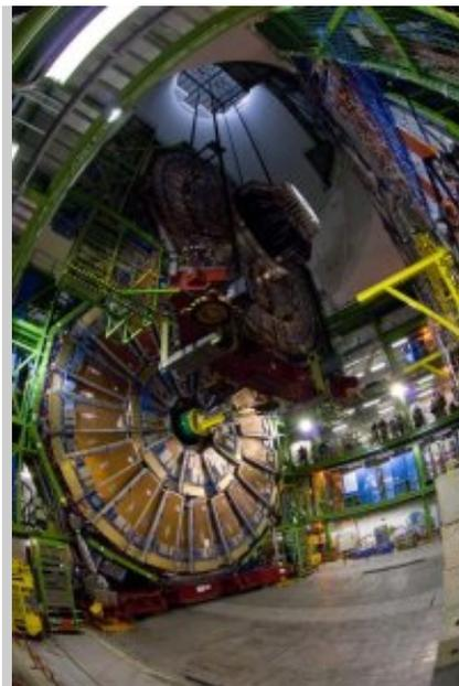
The final element of the Compact Muon Solenoid (CMS) detector at CERN descended into its underground experimental cavern on 22 January for the start-up of the Large Hadron Collider this summer. Future ILC detectors probably face a similarly spectacular descent - like CMS they will be assembled in a surface hall before they are transported to their cavern deep underground. Image courtesy of CERN. Read the [press release](#)
