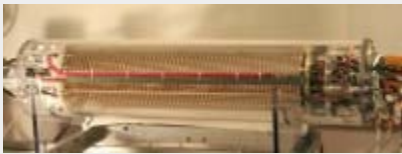
Cornell/Purdue small time projection chamber (TPC) prototype (LEPP, Cornell)
