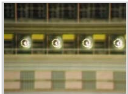
Top and side views of double stacked gold bumps. The pitch is 200 \mu\text{m} , the bump diameter is approximately 58 \mu\text{m} and the bump height is about 66 \mu\text{m} .
