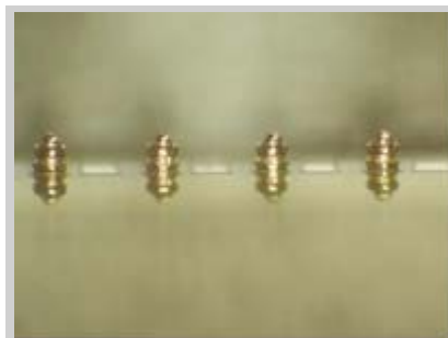
Top and side views of double stacked gold bumps. The pitch is 200 \mu\text{m} , the bump diameter is approximately 58 \mu\text{m} and the bump height is about 66 \mu\text{m} .
